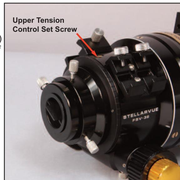
**Upper Tension Control:** There is an upper tension control that applies additional pressure to the drawtube and makes it more stable especially when imaging with a heavy camera. This tension control may be a set screw as shown or a thumb screw. Tighten this screw very slightly if needed to stabilize the drawtube. Use this adjustment screw only when necessary.
