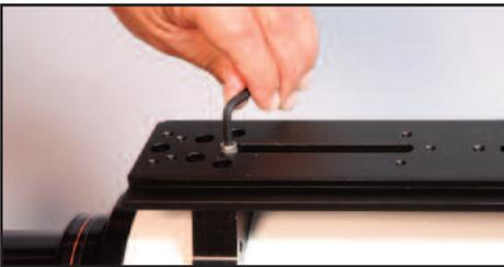
Screw the rail securely to the bottom of the rings. Vixen rails use one screw per ring, Losmandy rails use either one or two screws per ring. Using two screws in one ring and one in the other as shown in the picture to the left will securely hold the telescope in place.
