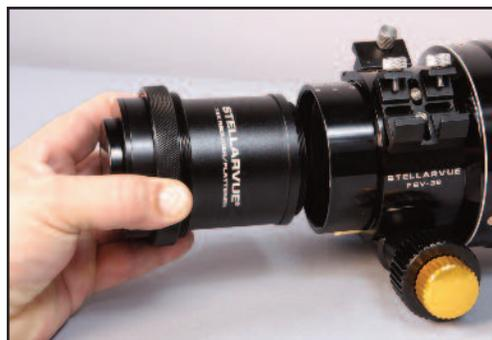
*Once the knurled focuser adapter is removed, take the SFFR.74 Reducer/Flattener and insert into the open end of the draw-tube of the focuser. Thread into the focuser draw-tube by turning clockwise. Once the Reducer/Flattener is securely hand-tightened, this conversion is complete.*
