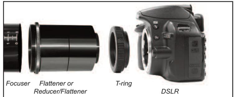
With other CCD cameras, the backfocus distances vary. Check with the maker of the camera to determine the backfocus of your camera. If the distance is less than 55 mm you will need to add extension tubes and/or spacer rings to make up the difference. For example, if your camera has a 35 mm backfocus you will need 20 mm of extension tubes to get the flattener 55 mm from the sensor in the camera.
