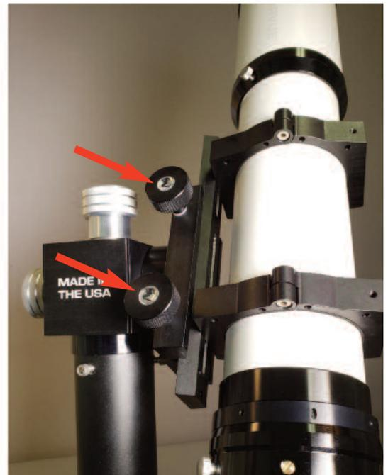
**Step 3:** Tighten the knob(s) securely.
