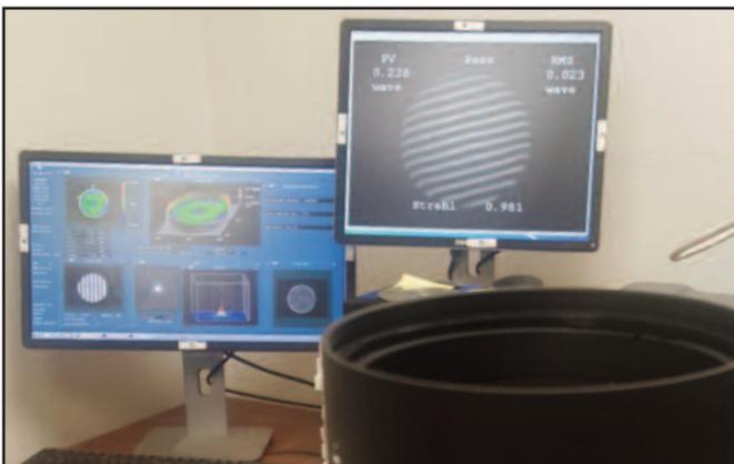
Stellarvue strives to ensure the highest optical accuracy. While many companies producing mass-produced lenses rely solely on test plates, we confirm the accuracy of each optical surface using our Zygo phase-shifting laser interferometer and extremely high precision test spheres that measure the entire clear aperture of the objective lens.
