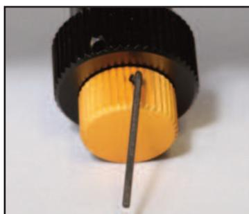
**Focus Knobs:** If there is a little play in the focusing knobs, use the supplied Allen wrench and tighten the set screw in the knob with play. This will fix the problem.
