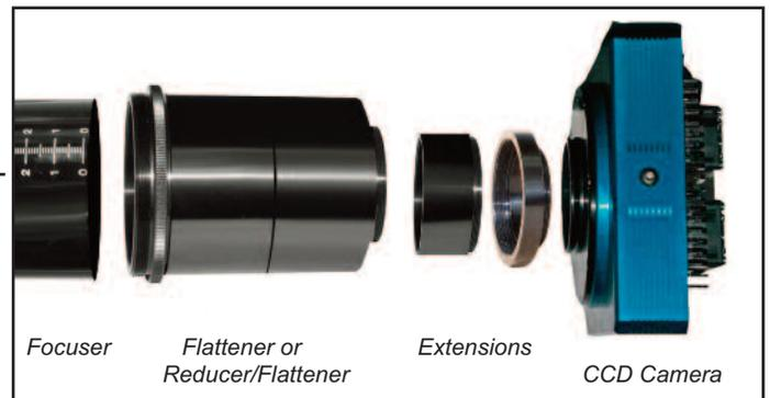
Telescopes vary in focal length slightly. This may have an impact on the necessary spacing between the field flattener and the ccd sensor. For this reason, astro-imagers generally have a collection of spacer rings and extension tubes so they can vary the distance slightly between a flattener or flattener/reducer and their camera to optimize the spacing.
