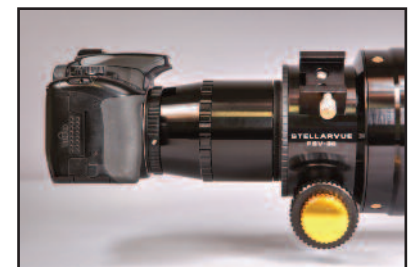
STEP 4: Thread the flattener to the drawtube & camera to flattener.
