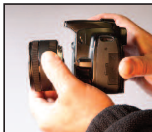
STEP 1: Remove the camera lens
