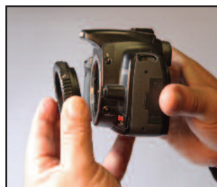
STEP 2: Install an oversized (48 mm) t-ring
