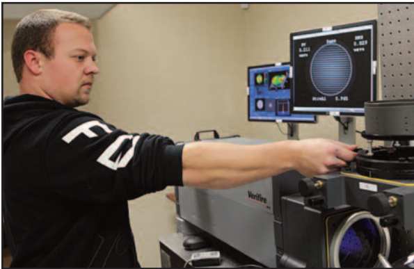
Alex our Production Manager using Stellarvue's Zygo Phase Shifting Laser Interferometer to test and adjust a Stellarvue Objective lens.
