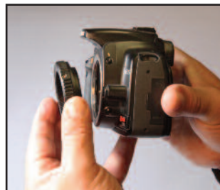
STEP 2: Install an oversized (48 mm) t-ring
