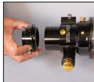
STEP 3: Unthread the 2" adapter from the focuser drawtube
