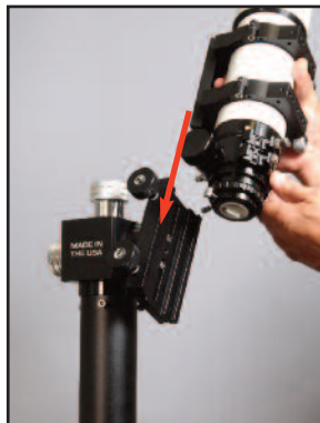
Step 2: Slide the mounting rail into the shoe.
