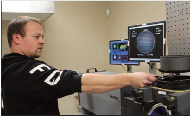
Alex our Production Manager using Stellarvue's Zygo Phase Shifting Laser Interferometer to test and adjust Stellarvue objectives.
