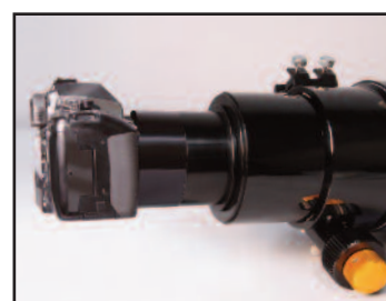
STEP 4: Thread the flattener to the drawtube & camera to flattener.
