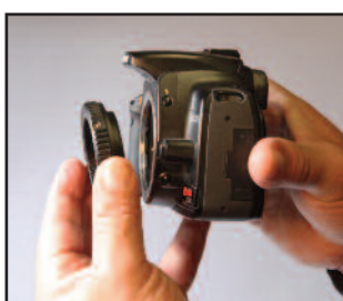
STEP 2: Install an oversized (48 mm) T-ring
