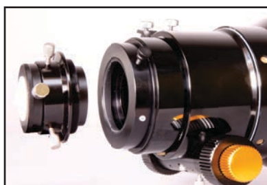
STEP 3: Unthread the 1 1/4" and 2" adapters from the focuser but leave the rotator in place.
