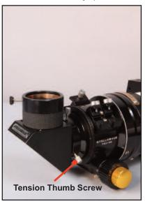
Install the diagonal and make sure it is held in place tight by tightening the tension thumb screws (all 3).
