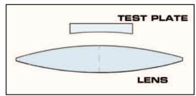
lens matches the curve on the test plate, straight lines will show under an intense testing light. Placing these glass plates on the surface of the lens may result in some very fine cosmetic lines or marks which do not affect performance in any way. This is normal in a high Strehl lens that is continually tested during polishing.
