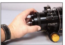
Now attach your camera to the flattener/reducer. If your system needs extension tubes or spacer rings, place them in between the camera and the reducer/flattener.
