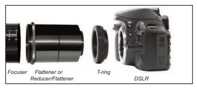
With other CCD cameras, the backfocus distances vary. Check with the maker of the camera to determine the backfocus of your camera. If the distance is less than 55 mm you will need to add extension tubes and/or spacer rings to make up the difference. For example, if your camera has a 35 mm backfocus you will need 20 mm of extension tubes to get the flattener 55 mm from the sensor in the camera.
